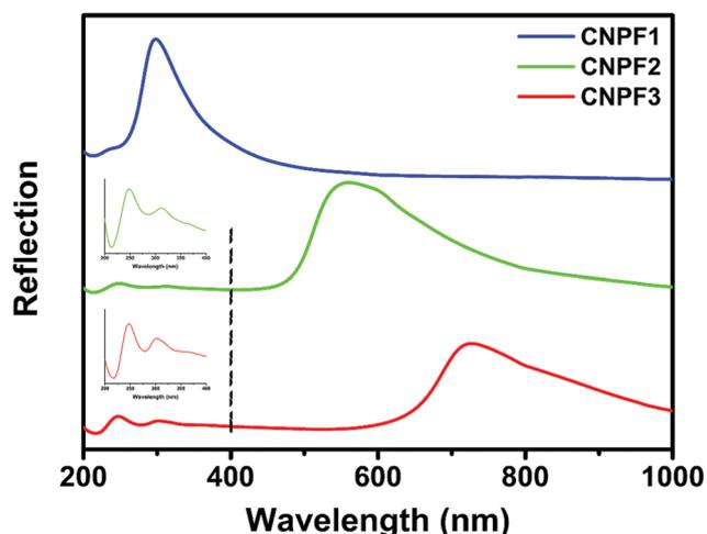
**Fig. 3** UV-Vis spectra of CNPF1–3 at normal incidence with varying photonic–photonic coupling. The inset shows the magnified UV spectra of CNPF2 and 3 at a short wavelength (200–400 nm) which highlights the surface grating induced double-peak spectra.
