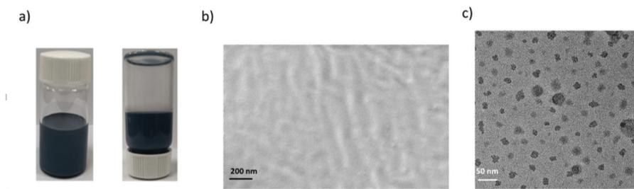
**Fig. 5** (a) Photograph of the composite dispersion in a transparent vial after standing for 20 d; (b) cross section SEM image of the fracture surface for the composite coating; and (c) TEM image of the composite dispersion.
