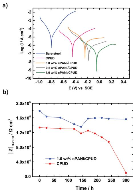
**Fig. 6** (a) PDP curves for bare steel, pure CPUD and composite coatings in 3.5 wt% NaCl solution; and (b) plots of  $|Z|_{0.01 \text{ Hz}}$  against the immersion time for pure CPUD and the 1.0 wt% cPANI/CPUD composite coating.
