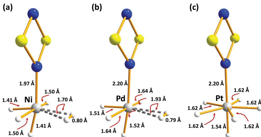
Fig. 5 B3LYP/6-31G(d,p) optimised structures of  $\text{H}_2$ -absorbed metal-doped  $\text{S}_2\text{N}_2$  (a)  $M = \text{Ni}$  (b)  $M = \text{Pd}$  (c)  $M = \text{Pt}$  (redrawn from computational data in ref. 35).
