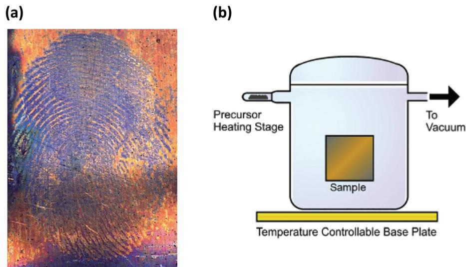
**Fig. 3** (a) Formation of  $(\text{SN})_x$  over latent fingerprints on metallic surfaces<sup>9c</sup> (reproduced with permission from S. M. Bleay, P. F. Kelly, R. S. B. King, *J. Mater. Chem.*, 2010, 20, 10100–10102. © 2010 The Royal Society of Chemistry.). (b) Diagram of  $\text{S}_2\text{N}_2$  processing equipment<sup>9d</sup> (reprinted with permission from S. M. Bleay, P. F. Kelly, R. S. P. King and S. G. Thorngate, *Sci. Justice*, 2019, 59, 606–621. © 2019 Elsevier B. V.).
