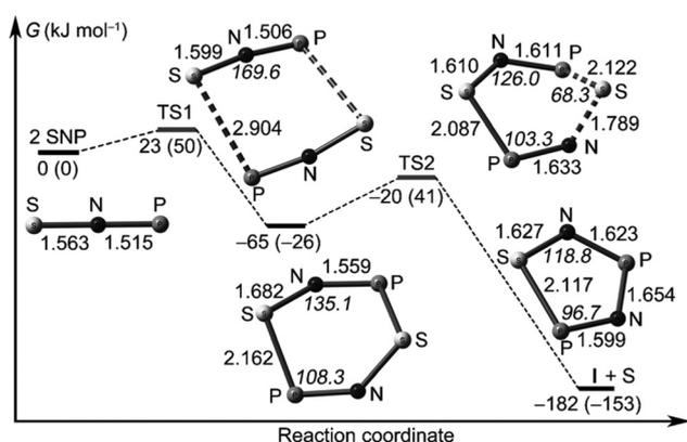
Fig. 12 Head-to-tail dimerisation of SNP and subsequent formation of *cyclo*-SNPNP; relative energies ( $\text{kJ mol}^{-1}$ ) and computed bond lengths ( $\text{\AA}$ ) at the B3LYP/6-311+G(3df) level.<sup>13</sup> (Reproduced with permission from X. Zeng, H. Li, H. Sun, H. Beckers, H. Willner and H. F. Schaefer III, *Angew. Chem., Int. Ed.*, 2015, **54**, 1327–1330. © 2015 WILEY-VCH Verlag GmbH & Co. KGaA, Weinheim.)
