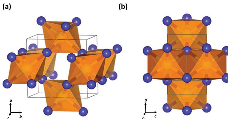
**Fig. 8** Crystal structure of  $\text{SN}_2$  formed at 81.6 GPa showing (a) the cross-linked octahedra and (b) the edge-sharing octahedra and apical S–N bonds.<sup>40</sup> (Reproduced with permission from D. Laniel, M. Bykov, T. Fedotenko, A. V. Ponomareva, I. A. Abrikosov, K. Glazyrin, V. Svitlyk, L. Dubrovinsky and N. Dubrovinskaja, *Inorg. Chem.*, 2019, **58**, 9195–9204. © 2019 The American Chemical Society.)
