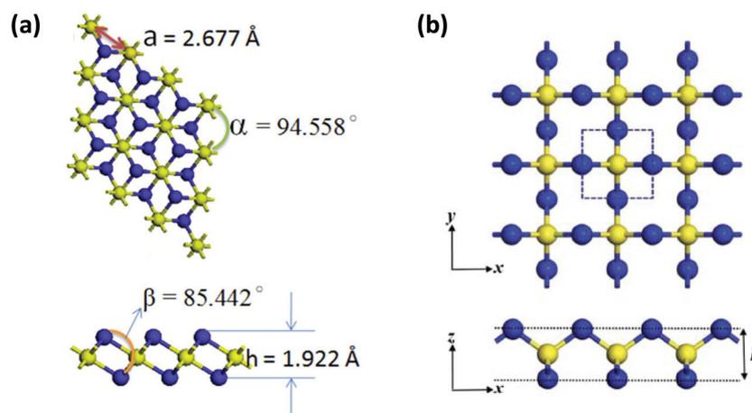
Fig. 6 Optimised structures of (a)  $1T\text{-SN}_2$ <sup>37</sup> (reproduced with permission from J.-H. Lin, H. Zhang, X.-L. Cheng and Y. Miyamoto, *Phys. Rev. B*, 2016, **94**, 195404. © 2016 American Physical Society), and (b)  $S\text{-SN}_2$ <sup>38</sup> (reproduced with permission from F. Li, X. Lv, J. Gu, K. Tu, J. Gong, P. Jin and Z. Chen, *Nanoscale*, 2020, **12**, 85–92. © 2020 The Royal Society of Chemistry).
