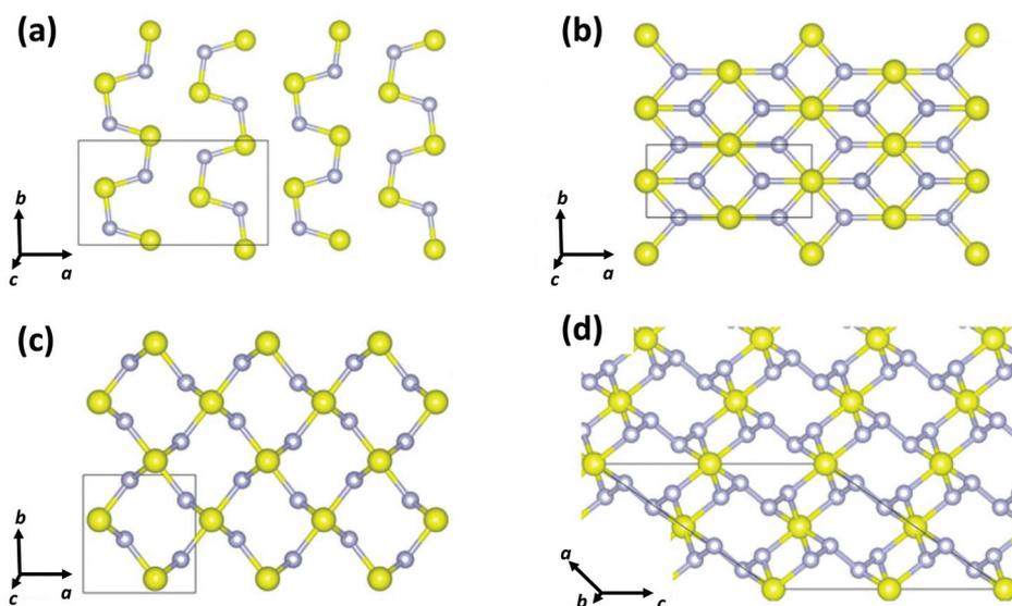
Fig. 7 Crystal structures of (a)  $Pnma$  ( $\text{SN}_x$ ), (b)  $Immm$  ( $\text{SN}_x$ ), (c)  $Pnmm$   $\text{SN}_2$ , and (d)  $C2/c$   $\text{SN}_4$ .<sup>39</sup> (Reproduced with permission from D. Li, F. Tian, Y. Z. Lv, S. Wei, D. Duan, B. Liu and T. Cui, *J. Phys. Chem. C*, 2017, **121**, 1515–1520. © 2017 The American Chemical Society.)
