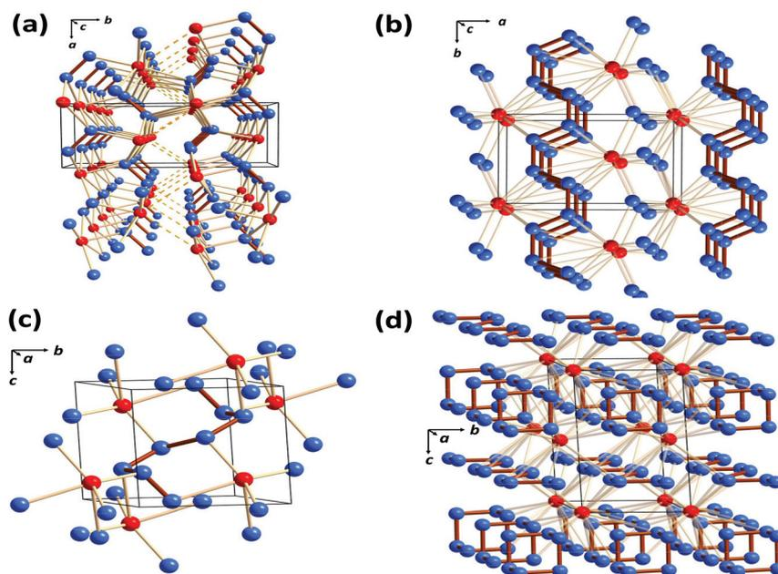
Fig. 9 Crystal structures of the predicted selenium nitrides: (a)  $Cmc2_1$ - $SeN_2$  at 90 GPa (b)  $P2_1/m$ - $SeN_3$  at 80 GPa (c)  $P\bar{1}$ - $SeN_4$  at 140 GPa and (d)  $P\bar{1}$ - $SeN_5$  at 130 GPa. Selenium atoms are depicted in red and nitrogen atoms in blue (redrawn from the structural data in ref. 52).
