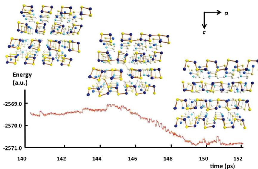
**Fig. 4** Simulated energy profile of the topochemical polymerisation of  $\text{S}_2\text{N}_2$  rings to  $(\text{SN})_x$  at 50 GPa and 600 K. Sulfur atoms are indicated by yellow spheres and nitrogen atoms by blue spheres ( $b$  axis is directed away from the reader).<sup>8</sup> (Reproduced with permission from T. T. Takaluoma, K. Laasonen and R. S. Laitinen, *Inorg. Chem.*, 2013, 52, 4648–4657. © 2013 American Chemical Society.)
