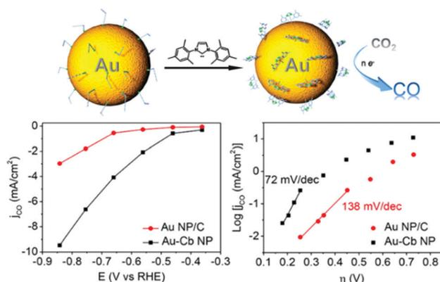
Fig. 35 Schematic illustration of NHC-carbene functionalized Au NPs for CO<sub>2</sub>RR to CO. Partial current density and Tafel plot for CO production for Au–Cb NP and Au NP/C. Reproduced with permission from ref. 454. Copyright 2016 American Chemical Society.
