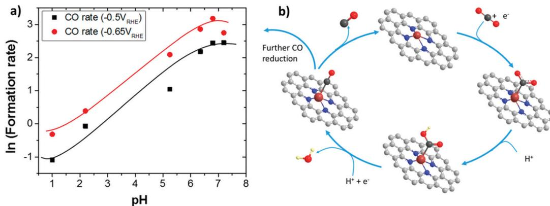
Fig. 25 (a) pH dependence of the CO formation rate at a constant potential on the RHE scale (black,  $-0.5 V_{\text{RHE}}$ ; red,  $-0.65 V_{\text{RHE}}$ ); (b) scheme of the proposed catalytic cycle of the  $\text{CO}_2\text{RR}$  on Fe-N-C catalysts. Adapted with permission from ref. 349. Copyright 2018 American Chemical Society.
