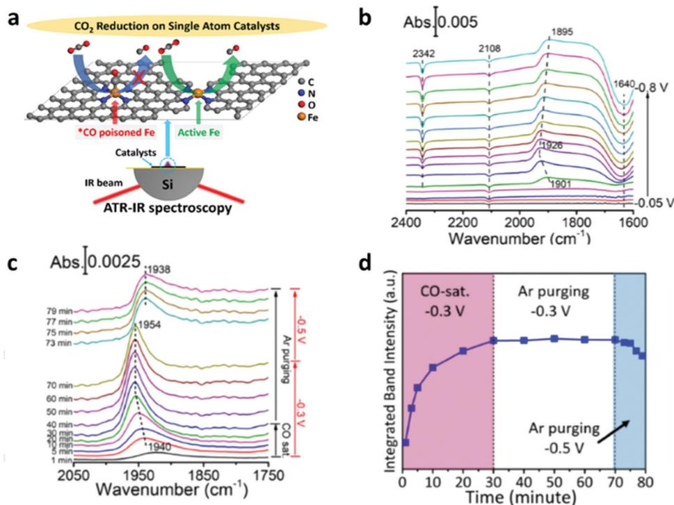
Fig. 23 (a) Scheme of the setup. (b) Real-time ATR-IR spectra recorded while stepping the potential of the Fe–N–C-loaded Au/Si prism in the CO<sub>2</sub>-saturated 0.5 M KHCO<sub>3</sub>. (c) Real-time IR spectra and (d) the evolution of the integrated \*CO band intensity when switching the CO/Ar atmosphere and potential. IR references were taken at 0 V for panel (b) and 0.1 V for panel (c). Adapted with permission from ref. 339. Copyright 2019 American Chemical Society.
