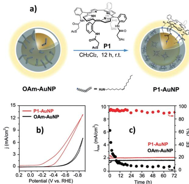
Fig. 32 (a) Synthesis of P1-Au NPs. (b) CV scans of OAm-Au NP and P1-Au NP electrodes under  $\text{CO}_2$ -saturated 0.5 M  $\text{KHCO}_3$  at pH 7.3. (c) Controlled-potential electrolysis of OAm-Au NP and P1-Au NP electrodes at  $-0.45$  V vs. RHE over a 72 h time course. Reproduced with permission from ref. 422. Copyright 2018 Wiley-VCH.
