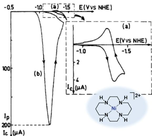
Fig. 13 Cyclic voltammetry of  $[\text{Ni}(\text{cyclam})]^{2+}$  (**40**, 1 mM) in 0.1 M  $\text{KClO}_4$  (pH 4.5) under  $\text{N}_2$  (curve a) or  $\text{CO}_2$  (curve b) on a hanging Hg electrode. Scan rate:  $0.1 \text{ V s}^{-1}$ . Reprinted with permission from ref. 210. Copyright 1986 American Chemical Society.
