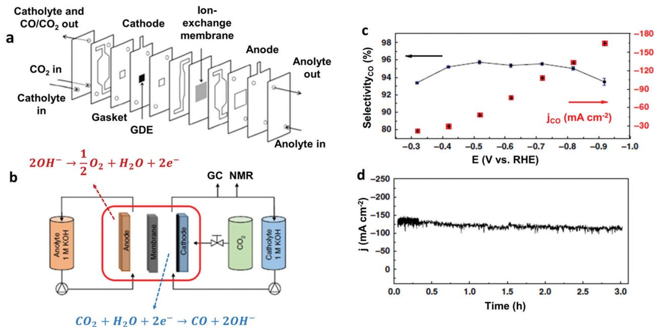
Fig. 11 (a) Cross-sectional view of the CO<sub>2</sub> electrolyzer flow cell and (b) general scheme of the entire experimental set-up used in ref. 186. (c) Current density (right) and selectivity for CO production (left) as a function of the potential, and (d) bulk electrolysis at a fixed potential ( $E = -0.72$  V vs. RHE) for **37**@carbon black deposited onto a carbon paper as cathodic material, in 1 M KOH. Adapted with permission from ref. 186. Copyright 2019, Nature Publishing Group.
