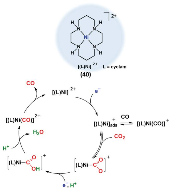
Scheme 2 Proposed mechanism for the electrochemical  $\text{CO}_2$ -to-CO catalyzed by  $[\text{Ni}(\text{cyclam})]^{2+}$  (**40**).<sup>210,215</sup>
