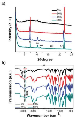
Fig. 4 (a) XRD patterns and (b) FT-IR spectra of self-assembled R-SPAn nanostructures formed in various mixed solvents. The drop-cast film of R-SPAn solution (THF) was used as 0% for these tests. [R-SPAn] = 1.5 mM. The diffraction peaks of the water fractions of 85% and 90% showed a body-centred cubic packing of the R-SPAn molecules. Upon increasing the water fraction from 0% to 90%, the FT-IR peaks ascribed to the stretching vibration of hydroxyl obviously shifted toward lower wavenumbers.
