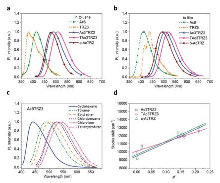
Fig. 3 Steady-state photophysical properties of the TSCT-HABs. PL spectra of the TSCT-HABs in toluene ( $10^{-5}$  mol L<sup>-1</sup>) (a) and in the film state (b), PL spectra of Ac3TRZ3 in solvents with different polarity (c), and the linear correlation of orientation polarization ( $\Delta f$ ) of the solvent with the Stokes shift for the TSCT-HABs (d) (see Table S1† for data).
