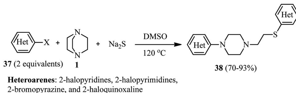
Scheme 12 Reaction of azaarene halides, DABCO, and Na<sub>2</sub>S for synthesis of piperazine derivatives.
