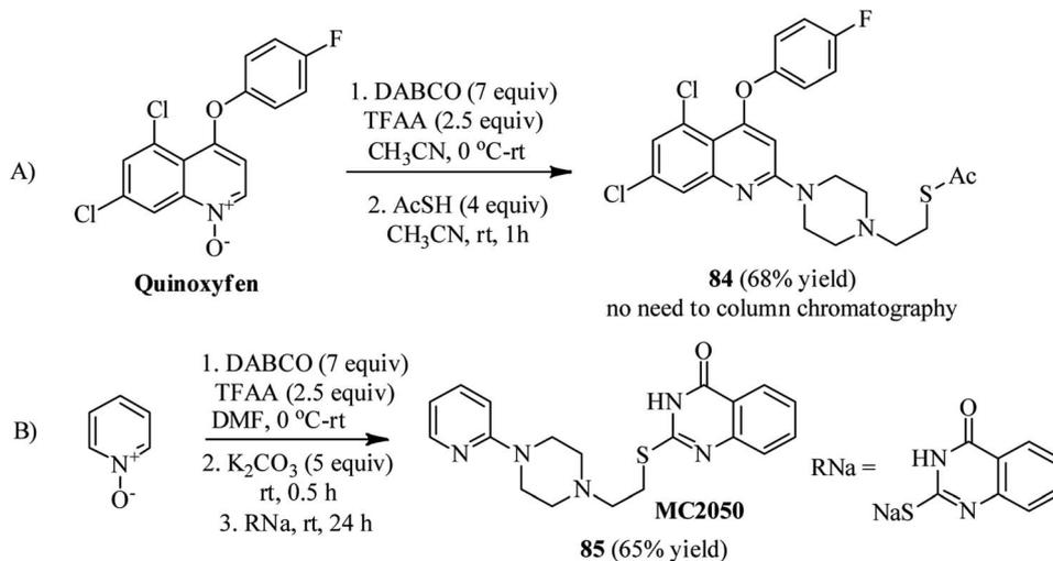
**Scheme 31** Synthesis of functionalized Quinoxifen-piperazine and MC2050 starting from pyridine-*N*-oxides.
