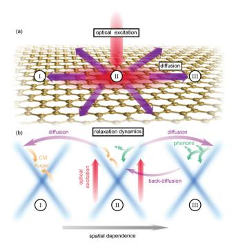
Fig. 1 Spatio-temporal carrier dynamics in graphene. (a) Optically excited carriers in spatial region II diffuse to regions I and III. (b) Many-particle scattering leads to relaxation in momentum space in each spatial region. Back-scattering *via* carrier–phonon processes and the resulting back-diffusion counteracts the spatial distribution of carriers.
