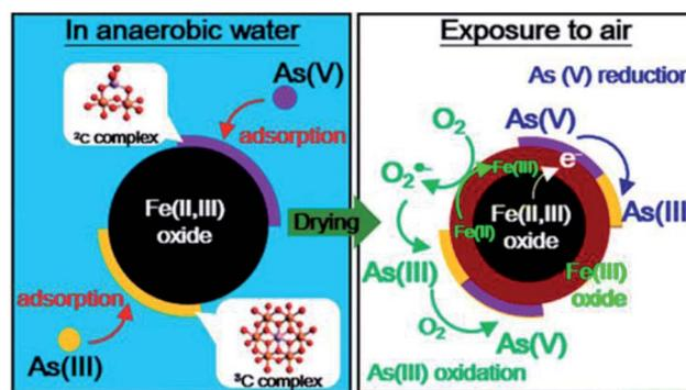
Fig. 7 Mechanism of arsenic adsorption on magnetite nanoparticles in anaerobic water and air-enriched water.<sup>190</sup>
