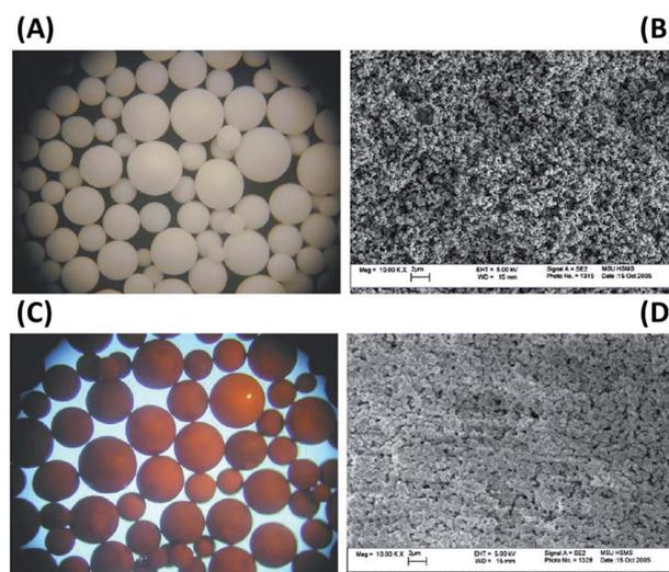
Fig. 6 (A) Light microscope photograph of SBA (45×); (B) SEM images of SBA and (C) light microscope photograph of HFO/SBA adsorbent (45×); (D) SEM images of HFO/SBA adsorbent.<sup>169</sup>
