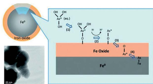
Fig. 8 The schematic diagram of the adsorption of As(III) species on nZVI particles.<sup>200</sup>
