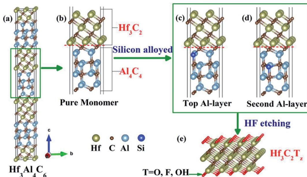
Fig. 2 Schematic illustration of the synthesis of  $Hf_3C_2T_x$  MXene from nanolaminated phase  $Hf_3[Al(Si)]_4C_6$ . (a) Structure of  $Hf_3Al_4C_6$ , (b) structure of pure  $Hf_3Al_4C_6$  monomer, (c) and (d) structure of two  $Hf_3Al_4C_6$  monomers with different silicon alloying, and (e) side view of  $Hf_3C_2$  MXene. Reprinted with permission of ref. 36 Copyright 2017 American Chemical Society.
