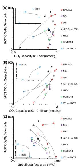
Fig. 10 Graphical "data mining" of the data shown in Table 1. CO<sub>2</sub>/N<sub>2</sub> selectivities (IAST or initial slope method) plotted versus (A) CO2 capacity at 1 bar, (B) CO<sub>2</sub> capacity at 0.1-0.15 bar, and (C) specific surface area of the adsorbents. SIFSIX samples are shown in the insets for comparison.
