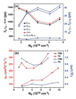
Fig. 6 (a) The contribution of different recombination channels  $(f_i\tau_i)$  in the case of the TIBr NCs is plotted against initial carrier density (twice the density of photons absorbed). (b) Effective carrier mobility (red) and carrier diffusion length (blue) for the (28.7 nm) TIBr and (8.4 nm) TII NCs, as a function of initial carrier density (fluence).
