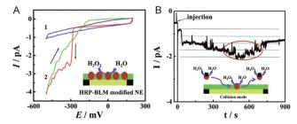
Fig. 5 Studying the single HRP with a BLM-Au nanoelectrode.  $^6$  (A) Cyclic voltammograms of the BLM-Au nanoelectrode (1) and HRP-embedded BLM-Au nanoelectrode (2) in a solution of 20 mM  $\rm H_2O_2$  and PBS buffer (pH: 7.4). (B) Chronoamperometric response of HRP collision into the BLM-Au electrode. Reproduced by permission of ref. 6 from The Royal Society of Chemistry.
