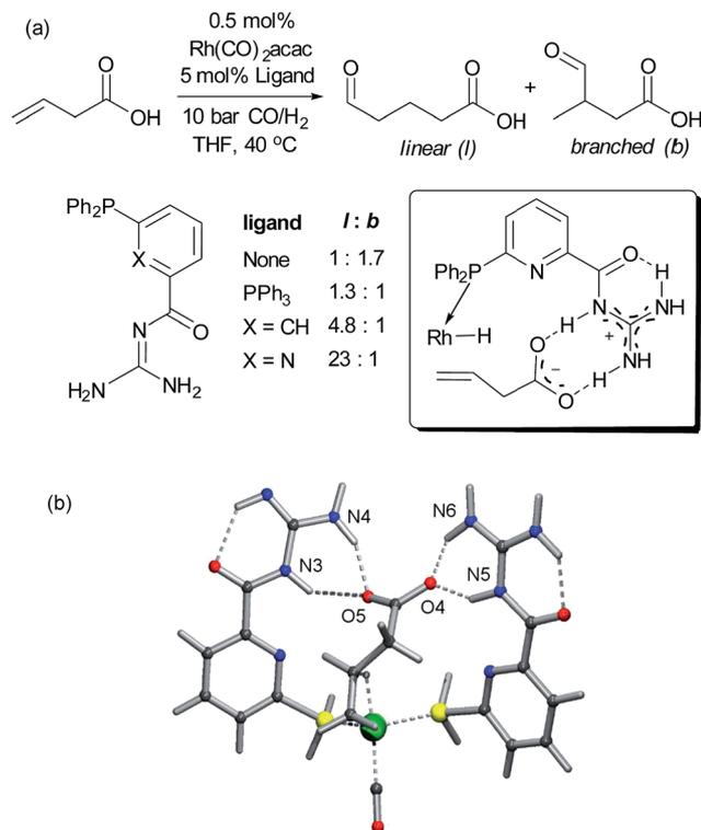
Fig. 7 (a) Evaluation of ligands for the hydroformylation of  $\beta,\gamma$ -unsaturated carboxylic acids and original hypothesis for control of regioselectivity. (b) Calculated transition state for reaction which involves interactions between two bifunctional ligands and the substrate. (b) Reprinted with permission from ref. 53. Copyright 2010 Wiley.
