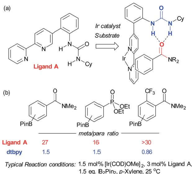
Fig. 3 (a) The optimal bifunctional bipyridine ligand bearing a hydrogen bond-donor urea, together with the catalyst–substrate complex thought responsible for *meta*-selective borylation. (b) A selection of substrates, highlighting *meta:para* selectivity for both the optimal bifunctional ligand and standard borylation ligand dtbpy.
