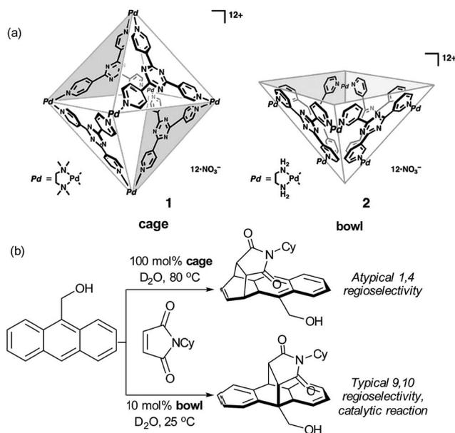
Fig. 5 (a) An octahedral cage and square-pyramidal bowl assembled from *cis* end-capped Pd(II) ions and triazine-cored tridentate ligands. (b) Divergent regioselectivity obtained in the presence of the cage and bowl structures in the Diels–Alder reaction of anthracenes with phthalimides. (a) Reprinted with permission from ref. 41. Copyright 2006 The American Association for the Advancement of Science.
