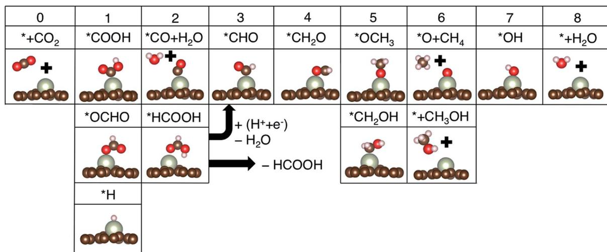
Fig. 3 Key reaction intermediate species for the CO<sub>2</sub> reduction reaction. The numbers on top of each column are the numbers of proton–electron pairs (H<sup>+</sup> + e<sup>-</sup>) transferred to CO<sub>2</sub>.
