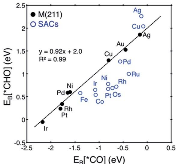
Fig. 5 Correlation between  $E_B[*CO]$  and  $E_B[*CHO]$  for transition metal (211) surfaces (black) vs. SACs (blue). The conventional scaling relation for M (211) is broken in the case of SACs. We note that Au@dv-Gr is not shown since it does not bind \*CO.
