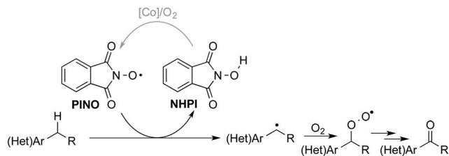
Scheme 3 Simplified mechanism depicting C–H abstraction by phthalimido-*N*-oxyl (PINO) and radical oxygenation by O<sub>2</sub>.
