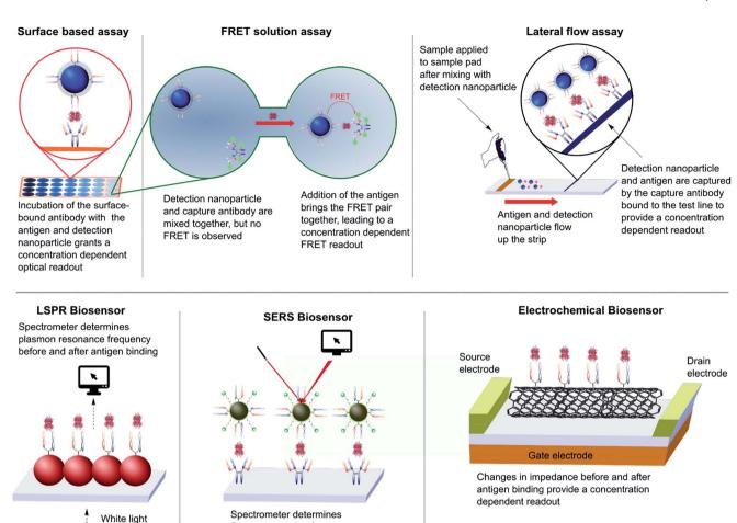
Fig. 7 Various designs of immunoassay ranging from surface based, FRET and lateral flow assays to LSPR, SERS and electrochemical biosensing.
