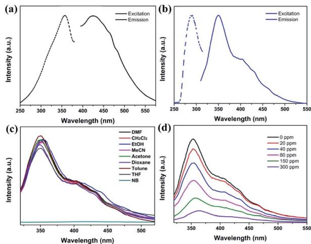
Fig. 2 Excitation (dot lines) and emission (solid lines) spectra of the free H<sub>3</sub>TATMA ligand (a) and 1 dispersed in DMF (b). (c) Luminescent intensity of 1 crystal powder after immersing in DMF with 600 ppm of different analytes for about 2 minutes at room temperature upon excitation at 292 nm. (d) The emission spectra of 1 titrated with NB in DMF for about 2 minutes. 4.0 mg of 1 crystal powder was dispersed in 3.0 mL DMF.
