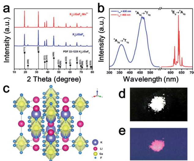
Fig. 1 (a) XRD patterns of  $K_2LiGaF_6$  and  $K_2LiGaF_6:Mn^{4+}$ , (b) PLE and PL spectra of  $K_2LiGaF_6:Mn^{4+}$ , (c) structure diagram, (d) phosphor under natural light and (e) phosphor under UV-light.
