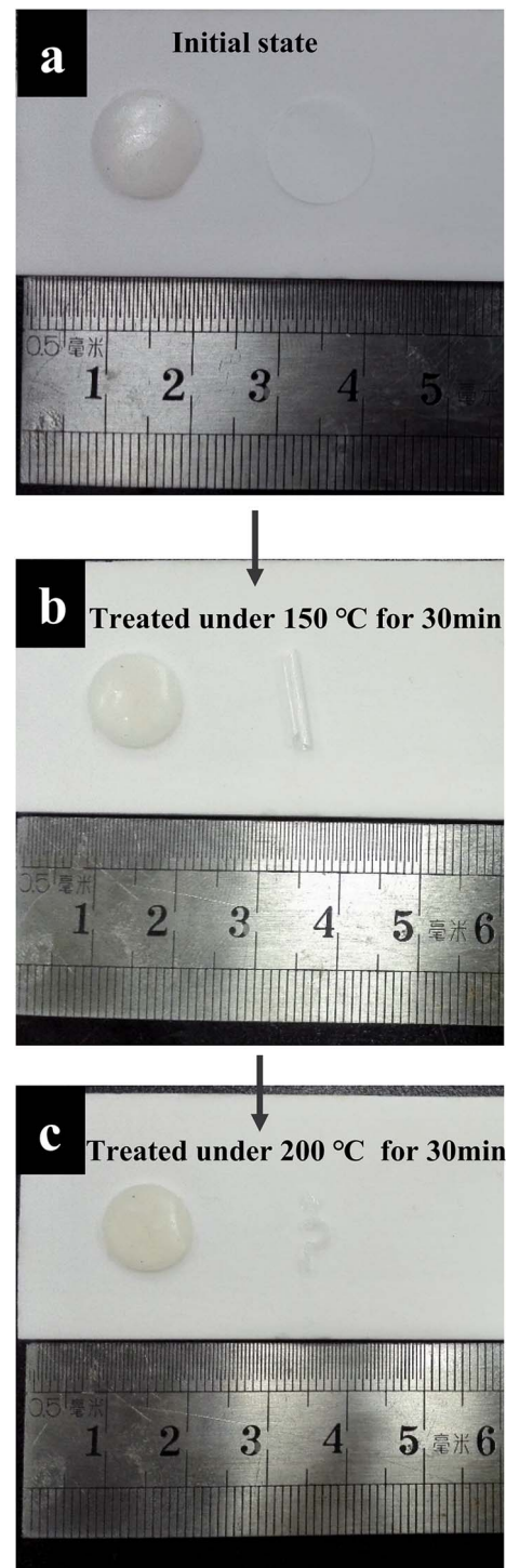
Fig. 2 Photo image of GPE and commercial separator (a) initial state, (b) heat treatment at 150 °C for 30 min and (c) further heat treatment at 200 °C for 30 min.
