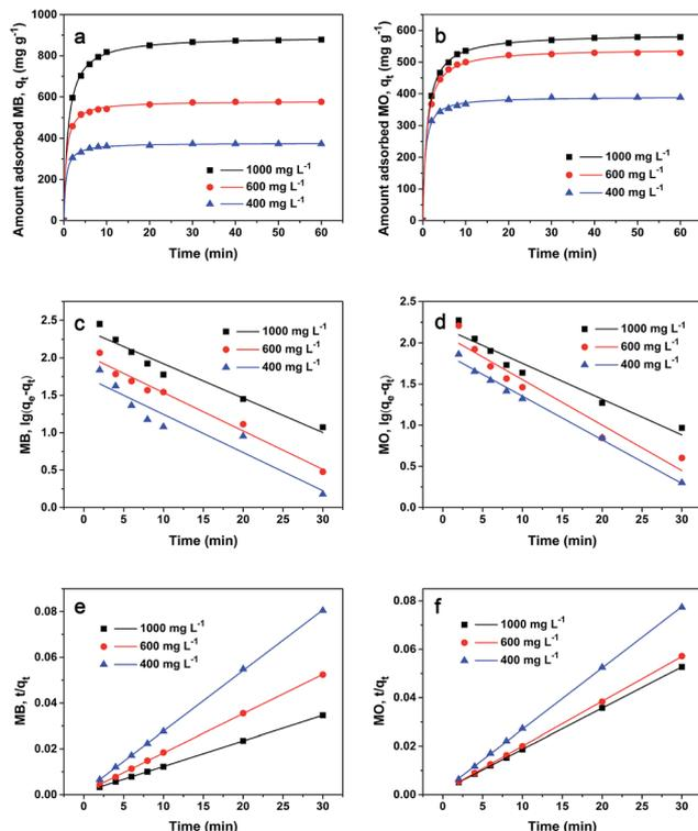
Fig. 3 Adsorption capacity of (a) MB and (b) MO as a function of time at different initial concentrations. Linear regressions of (c) MB and (d) MO according to pseudo-first-order kinetic model. Linear regressions of (e) MB and (f) MO according to pseudo-second-order kinetic model.
