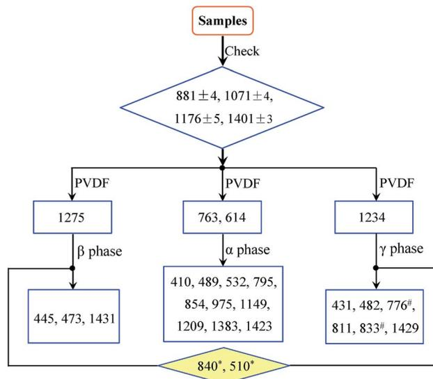
Fig. 1 Flow diagram for the identification of α, β and γ phases; 840\* and 510\* represents bands in the range of 837–841 and 508–512 cm<sup>-1</sup>, respectively; 776# and 833# reflects possible variations based on specific processes.
