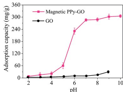
Fig. 8 Adsorption capacities of GO and magnetic PPy-GO under various pH conditions. Conditions:  $T = 300 \text{ K}$ ,  $\text{RSL} = 0.05 \text{ g L}^{-1}$  and  $C_0 = 20 \text{ mg L}^{-1}$  for magnetic PPy-GO;  $T = 298 \text{ K}$ ,  $\text{RSL} = 0.5 \text{ g L}^{-1}$  and  $C_0 = 100 \text{ mg L}^{-1}$  for GO.<sup>32</sup>
