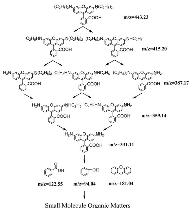
**Scheme 1** Proposed degradation pathway of photocatalytic degradation of RhB by ZnIn<sub>2</sub>S<sub>4</sub> under visible light irradiation.
