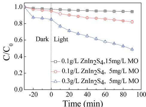
Fig. 2 Photocatalytic degradation of MO with different  $\text{ZnIn}_2\text{S}_4$  dosage ( $0.1 \text{ g L}^{-1}$  or  $0.3 \text{ g L}^{-1}$ ) and initial concentration of MO ( $15 \text{ mg L}^{-1}$  or  $5 \text{ mg L}^{-1}$ ).
