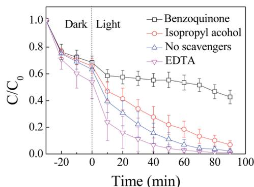
Fig. 4 Photocatalytic degradation of RhB by  $\text{ZnIn}_2\text{S}_4$  under visible light irradiation in the presence of scavengers: EDTA, benzoquinone, and isopropyl alcohol were used to capture holes,  $\text{O}_2^-$ , and  $\cdot\text{OH}$ , respectively.
