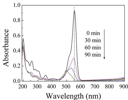
Fig. 5 UV-Vis spectra of degraded RhB solution under visible light irradiation with an initial RhB concentration of  $15 \text{ mg L}^{-1}$  and a  $\text{ZnIn}_2\text{S}_4$  dosage of  $0.1 \text{ g L}^{-1}$ .
