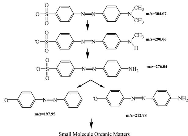
**Scheme 2** Proposed degradation pathway of photocatalytic degradation of MO by ZnIn<sub>2</sub>S<sub>4</sub> under visible light irradiation.
