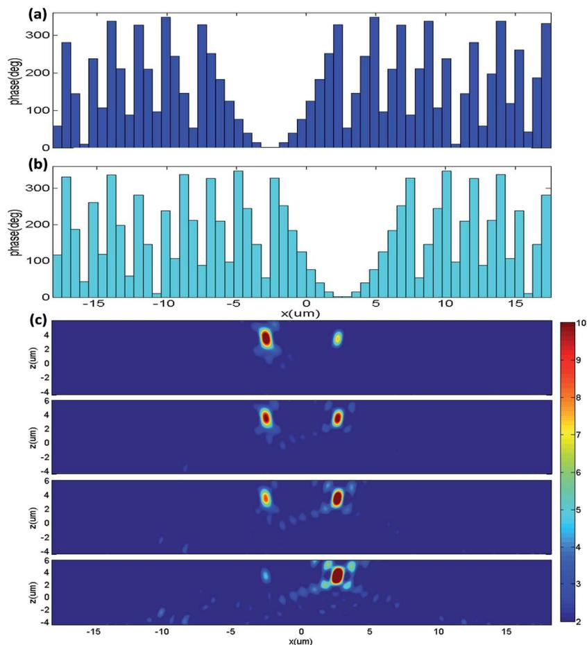
Fig. 5 (a) The required transmitted phase along  $x$ -axis when incidenting  $x$ -polarized and (b)  $y$ -polarized light to realize the function of focus. (c) Transmitted intensity distributions of the metasurface illuminated with a normal LP incidences with polarization-angle of  $30^\circ$ ,  $38^\circ$ ,  $45^\circ$  and  $60^\circ$ , respectively.
