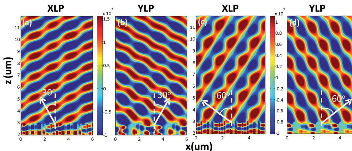
Fig. 3 Transmitted XLP (a and c) and YLP (b and d) electric field distributions of the metasurface illuminated with a normal incidences of  $45^\circ$  LP lights with the refractive angles of  $30^\circ$  (a and b) and  $60^\circ$  (c and d).
