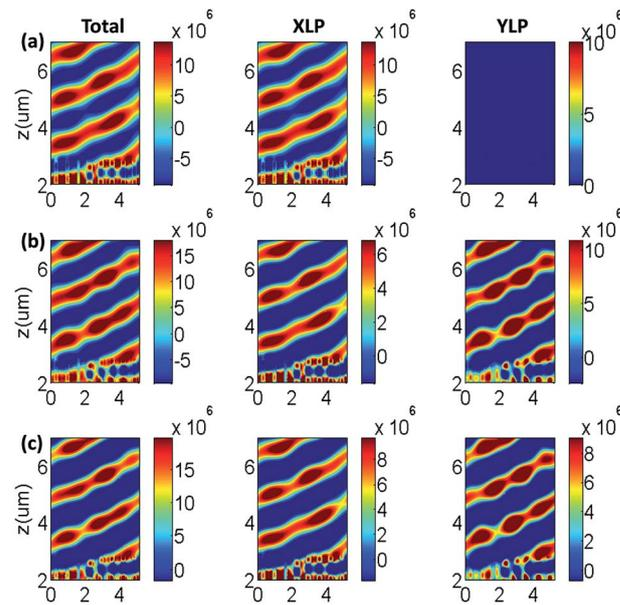
Fig. 4 Transmitted total, XLP and YLP electric field distributions of the metasurface illuminated with normal incidences of XLP light (a),  $30^\circ$  LP light (b) and  $45^\circ$  LP light (c) with the refractive angles of  $17^\circ$ .
