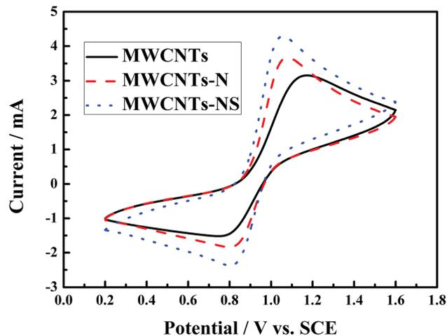
Fig. 3 Cyclic voltammograms of glassy carbon electrodes modified by different MWCNTs samples at the scan rate of  $20 \text{ mV s}^{-1}$  in a  $2.0 \text{ mol L}^{-1} \text{ VOSO}_4 + 3.0 \text{ mol L}^{-1} \text{ H}_2\text{SO}_4$  electrolyte solution.
