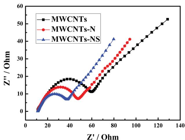
Fig. 4 Electrochemical impedance spectroscopy of glassy carbon electrodes modified by different MWCNTs samples in  $1.0 \text{ mol L}^{-1} \text{ VOSO}_4 + 3.0 \text{ mol L}^{-1} \text{ H}_2\text{SO}_4$  at open-circuit voltage.
