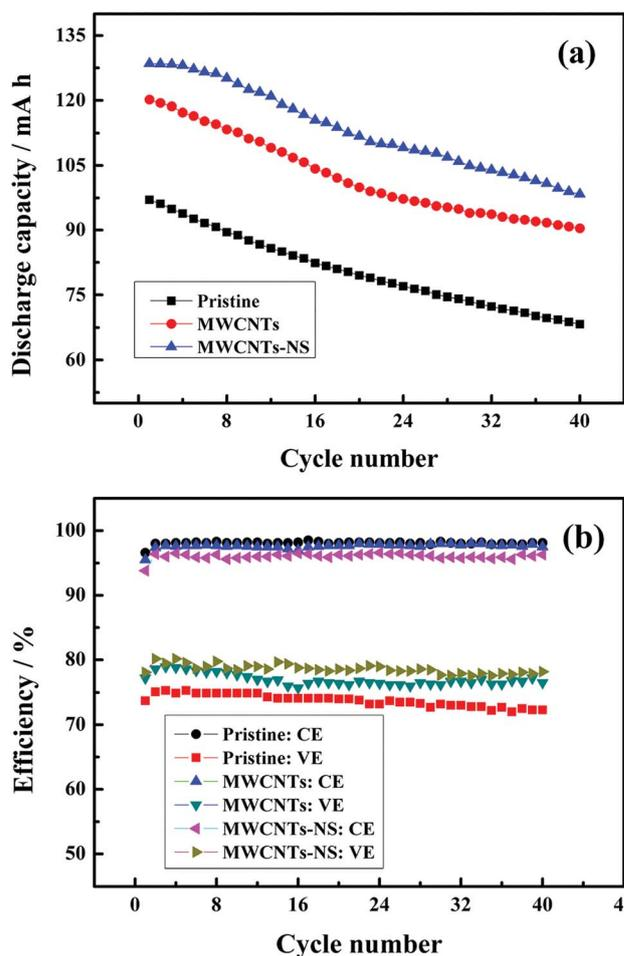
Fig. 7 The discharge capacity (a) and efficiency (b) of the cells using different MWCNTs samples as a function of cycle number at the current density of 50 mA cm<sup>-2</sup>.
