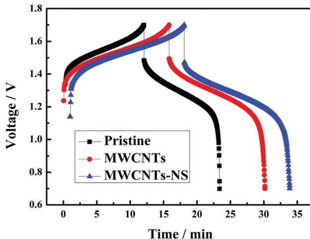
Fig. 6 The 10<sup>th</sup> charge–discharge curves of the cell using the MWCNTs samples as a catalyst in the positive side at a current density of 50 mA cm<sup>-2</sup>.
