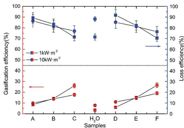
Fig. 6 The vaporization efficiency and loss efficiency of pure water and Au NPs dispersions with different diameters (sample A to F) under solar illumination with 1 and  $10 \text{ kW m}^{-2}$ , respectively.
