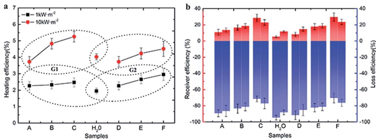
Fig. 8 Three kinds of efficiencies for photothermal conversion. (a) Heating efficiency of Au nanoparticles from G1 and G2 under 1 and  $10 \text{ kW m}^{-2}$  solar illumination. (b) Receiver efficiency and loss efficiency of Au nanoparticles from G1 and G2 under 1 and  $10 \text{ kW m}^{-2}$  illumination.
