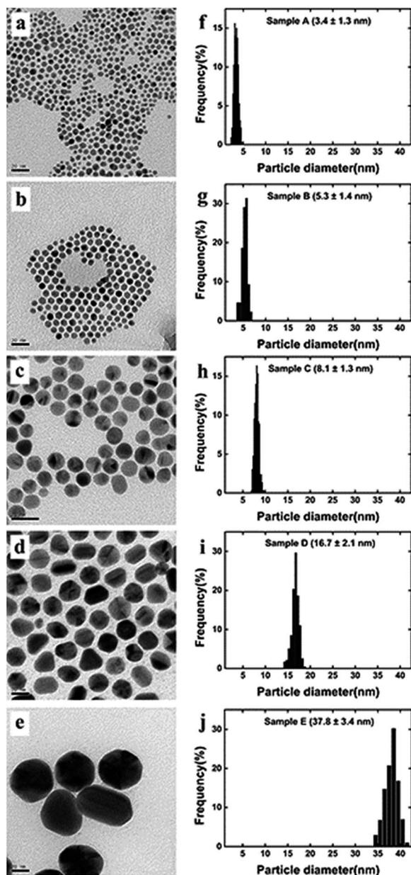
Fig. 3 TEM images and size distributions of gold nanoparticles: (a) and (f) for sample A ( $3.4 \pm 1.3$  nm), (b) and (g) for sample B ( $5.3 \pm 1.4$  nm), (c) and (h) for sample C ( $8.1 \pm 1.3$  nm), (d) and (i) for sample D ( $16.7 \pm 2.1$  nm) and (e) and (j) for sample e ( $37.8 \pm 3.4$  nm).
