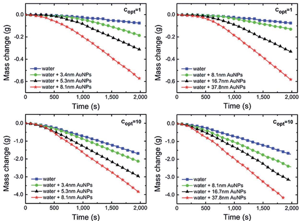
Fig. 5 The mass loss (evaporated water) of Au NPs dispersions with different diameters under 1 and 10 kW m<sup>-2</sup> xenon lamp's illumination compared with pure water. Au NPs from G1 (a) and G2 (b) were irradiated under 1 kW m<sup>-2</sup> illumination. Similarly, Au NPs from G1 (c) and G2 (d) were irradiated under 10 kW m<sup>-2</sup> illumination.
