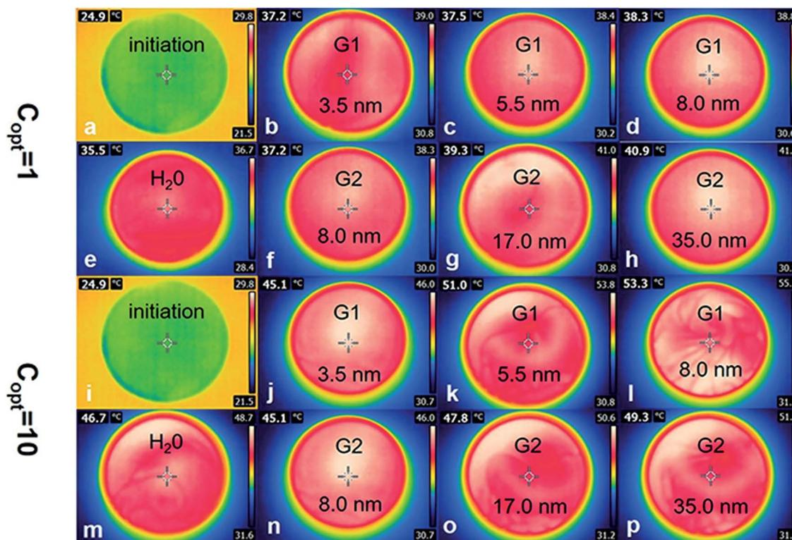
Fig. 7 The temperature of pure water and Au NPs nanofluids with different diameters before and after  $\sim 2000$  s solar illumination under  $1 \text{ kW m}^{-2}$  (a)–(h) and  $10 \text{ kW m}^{-2}$  solar illumination (i)–(p), respectively.
