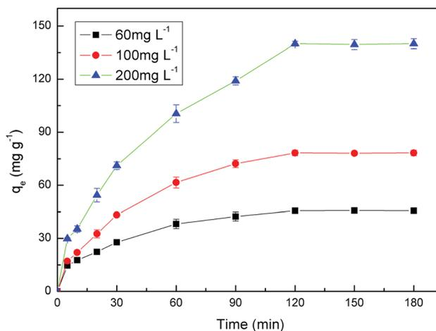
Fig. 7 Effect of contact time on  $U(VI)$  adsorption. (Volume, 30 mL; adsorbent dose, 0.03 g; initial concentration, 60, 100 and  $200\ mg\ L^{-1}$ ; pH value, 4.0; contact time, 0, 5, 10, 20, 30, 60, 90, 120, 150, 180 min; temperature,  $25\ ^\circ C$ ; rotating speed, 150 rpm.)
