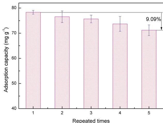
Fig. 11 Adsorption/desorption cycles (initial concentration: 100 mg L<sup>-1</sup>).
