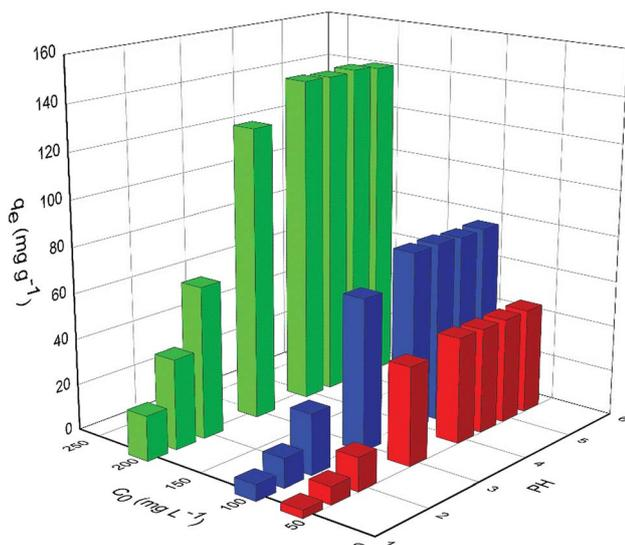
Fig. 5 The effect of initial solution pH on  $U(VI)$  removal by PAA hydrogels at various initial concentrations (60, 100 and  $200\ mg\ L^{-1}$ ). (Volume, 10 mL; adsorbent dose, 0.01 g; pH value, 1, 1.5, 2, 3, 4, 4.5, 5, 5.5; contact time, 180 min; temperature,  $25\ ^\circ C$ ; rotating speed, 150 rpm). Note: data are presented as the mean  $\pm$  standard deviation of triplicate experiments.
