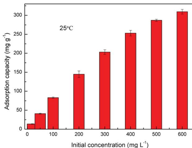
Fig. 6 The effect of initial concentrations (20, 50, 100, 200, 300, 400, 500,  $600\ mg\ L^{-1}$ ) on  $U(VI)$  removal by PAA hydrogels. (Volume, 10 mL; adsorbent dose, 0.01 g; pH value, 4.0; contact time, 180 min; temperature,  $25\ ^\circ C$ ; rotating speed, 150 rpm.)
