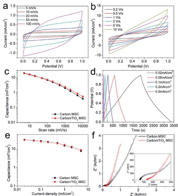
Fig. 4 Electrochemical properties of the carbon/TiO<sub>2</sub> composite electrode. CV curves at low scan rate (a) and high scan rate (b), specific capacitance calculated from CV data as a function of scan rate (c), CC curves (d), specific capacitance calculated from CC data as a function of current density (e), and Nyquist plots of MSCs before and after TiO<sub>2</sub> deposition (f). The inset in (f) shows the high-frequency region of the Nyquist plots.
