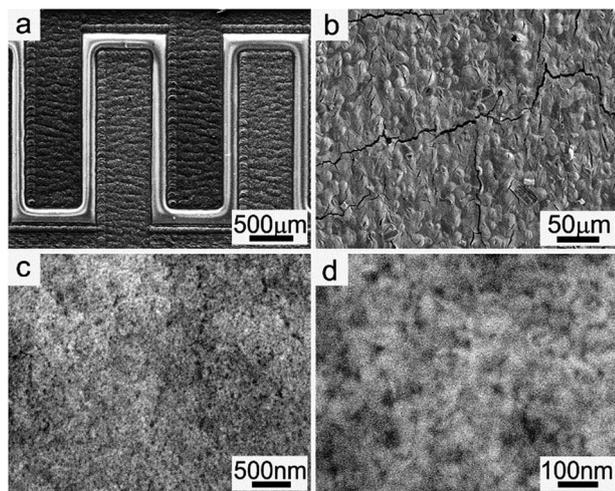
Fig. 2 Large-scale (a and b) and enlarged SEM images (c and d) of the carbon/TiO<sub>2</sub> composite electrode obtained by laser direct writing on PI film in Ar and following electrophoretic deposition of TiO<sub>2</sub> nanoparticles.
