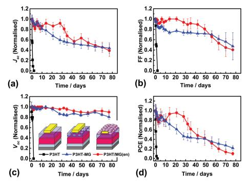
Fig. 6 (a) to (d) Normalised solar cell figures of merit for P3HT/MG(en) ( $C_{MG} = 3.0\%$ ), P3HT-MG and control P3HT PSCs exposed to 40% humidity at room temperature. The PSCs were stored in the dark between measurements. The legend from (c) also applies to (a), (b) and (d).
