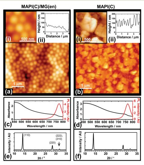
Fig. 5 AFM images and line-traces (a and b), UV-visible and PL spectra (c and d) and XRD data (e and f) for MAPI(C) encapsulated by an MG film (MAPI(C)/MG(en),  $C_{MG} = 4.6\%$ ) and an unmodified MAPI(C) film. The films were deposited on ITO/bl-TiO<sub>2</sub>.
