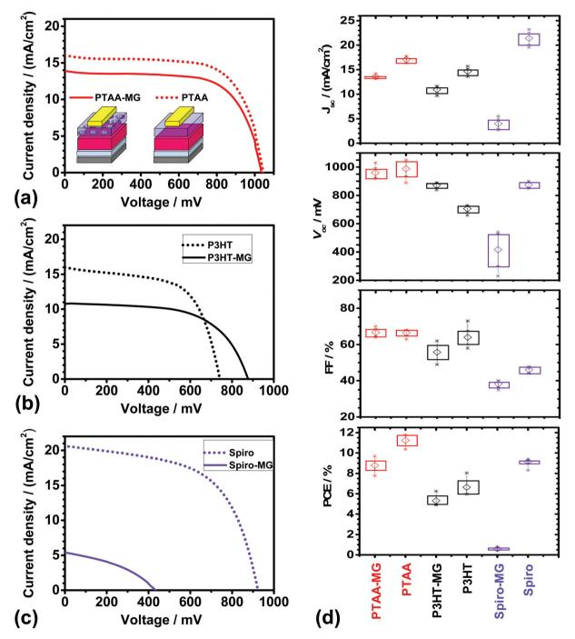
Fig. 3 J-V curves for PSCs with HTMs of (a) PTAA-MG or PTAA, (b) P3HT-MG or P3HT and (b) Spiro-MG or Spiro. (d) Solar cell metrics for the various PSCs. The average values are shown by the open symbols. The rectangles show the upper and lower values for the average  $\pm$  the standard deviation. The maximum and minimum values measured for each PSC are shown by the stars.
