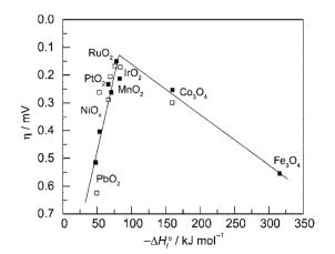
Fig. 3 Volcano plot showing activity for  $O_2$  production on metal oxide surfaces *versus* the enthalpy of transition of the oxide in acidic ( $\blacksquare$ ) and basic ( $\square$ ) solutions. Overpotential measured relative to 0.1 mA cm<sup>-2</sup> current density. Reprinted with permission.<sup>21</sup> Copyright 2010, American Chemical Society.
