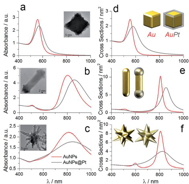
Fig. 2 Optical characterisation of the nanoparticles in solution. (a–c) Experimental and (d–f) simulated spectra of the bare gold (red) and Pt-coated (grey) nanoparticles with cubic (a, d), rod-like (b, e) and star-like morphology (c, f). Insets in (d–f) represent three-dimensional images of the particles used in simulations.
