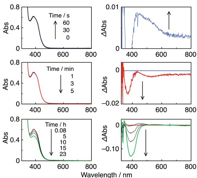
Fig. 9 UV-vis (left) and the corresponding differential absorption spectral changes (right) during the irradiation of a CO<sub>2</sub>-saturated DMA-TEOA (5 : 1 v/v) solution containing R(5) (0.05 mM) as the PS and Ru(*t*Bu)-Cl<sub>2</sub> (0.05 mM) as the catalyst, under irradiation at  $\lambda_{\text{ex}} = 436$  nm ( $4.2 \times 10^{-9}$  einstein per s).
