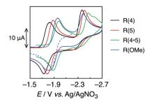
Fig. 2 Cyclic voltammograms of R(X) (0.5 mM) in DMF under Ar, measured with a 100 mV  $\rm s^{-1}$  sweep rate.
