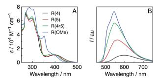
Fig. 1 UV-vis (A) and emission (B) spectra of the Re-rings in DMF under Ar. The emission spectra were corrected to the absorbed photons at  $\lambda_{\rm ex}=400$  nm.
