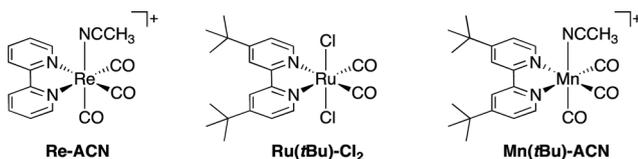
Chart 2 Structures and abbreviations of the Re(I), Ru(II) and Mn(II) catalysts. Re(I) and Mn(II) complexes were synthesized as  $\text{PF}_6^-$  salts.
