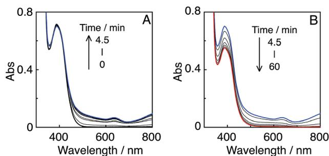
Fig. 11 UV-vis absorption spectral changes of a CO<sub>2</sub>-saturated DMA-TEOA (5 : 1 v/v) solution containing R(5) (0.05 mM) as the PS and Mn(tBu)-ACN (0.05 mM) as the catalyst, under irradiation at  $\lambda_{\text{ex}} = 436$  nm ( $5.3 \times 10^{-9}$  einstein per s) in the initial stage (A) and over 1 h irradiation (B).
