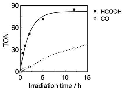
Fig. 10 Photocatalytic CO<sub>2</sub> reduction using R(5) (0.05 mM) as the PS and Mn(tBu)-ACN (0.05 mM) as the catalyst in DMA-TEOA (5 : 1 v/v) under 436 nm light irradiation of  $5.3 \times 10^{-9}$  einstein per s intensity.
