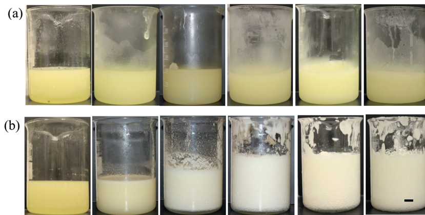
Fig. 5 Photographs of vessels containing mixtures of MA in HOSO at different concentrations (a) before aeration and (b) immediately (within 1 min) after whipping at 22 °C. MA concentrations in wt% are (left to right) 2.0, 3.5, 4.5, 5.0, 6.0 and 10.0. The sample at 2.0 wt% is one-phase, all other samples are two-phase. Scale bar = 1 cm.
