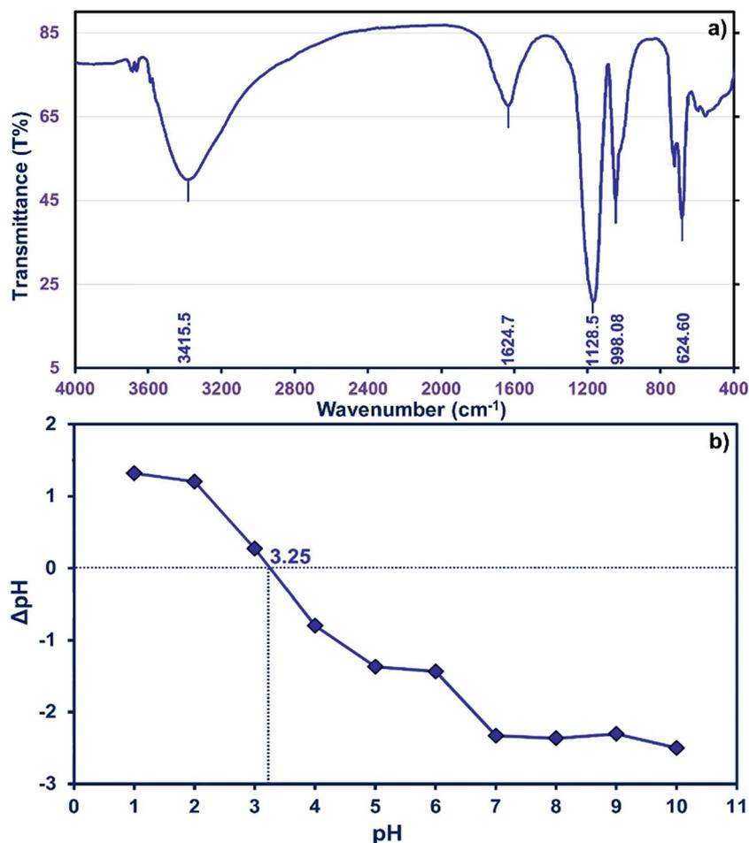
Fig. 2 (a) FTIR spectrum and (b)  $pH_{zpc}$  obtained from ZnS-NP-AC.
