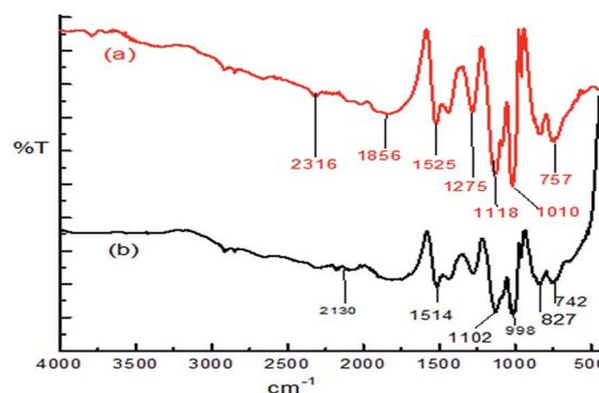
Fig. 1 The FTIR spectra of the PPy before (a) and after (b) the adsorption of nickel.<sup>97</sup>
