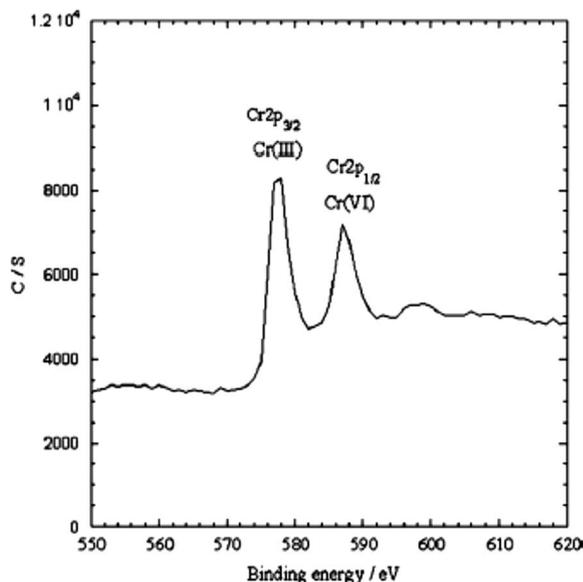
Fig. 4 The XPS spectra of the PPy/Fe<sub>3</sub>O<sub>4</sub> nanocomposites after Cr(vi) adsorption.<sup>113</sup>
