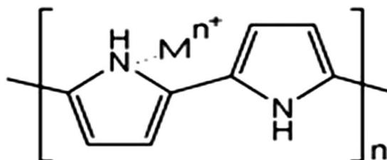
Scheme 1 A plausible mechanism for metal ion adsorption on the surface of nitrogen functional groups in PPy conducting polymer.<sup>97</sup>
