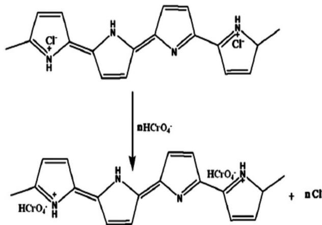
Scheme 3 A plausible mechanism for the removal of Cr(II) ions from aqueous solution.<sup>113</sup>
