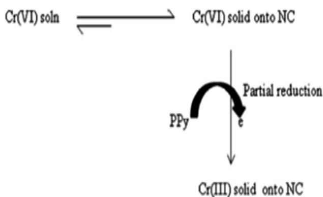
Scheme 5 The mechanism for adsorption and partial reduction of  $\text{Cr(VI)}$  onto the PPy-OMMTC nanocomposite.<sup>123</sup>
