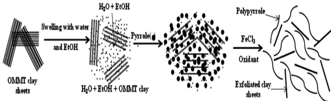
Fig. 7 The formation of exfoliated PPy-OMMTC nanocomposites.<sup>123</sup>
