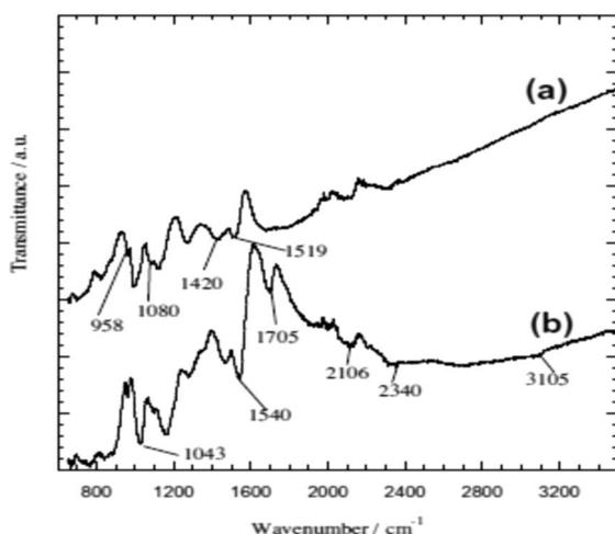
Fig. 2 The ATR-FTIR spectra of (a) PPy homopolymer and (b) PPy-gly.<sup>38</sup>
