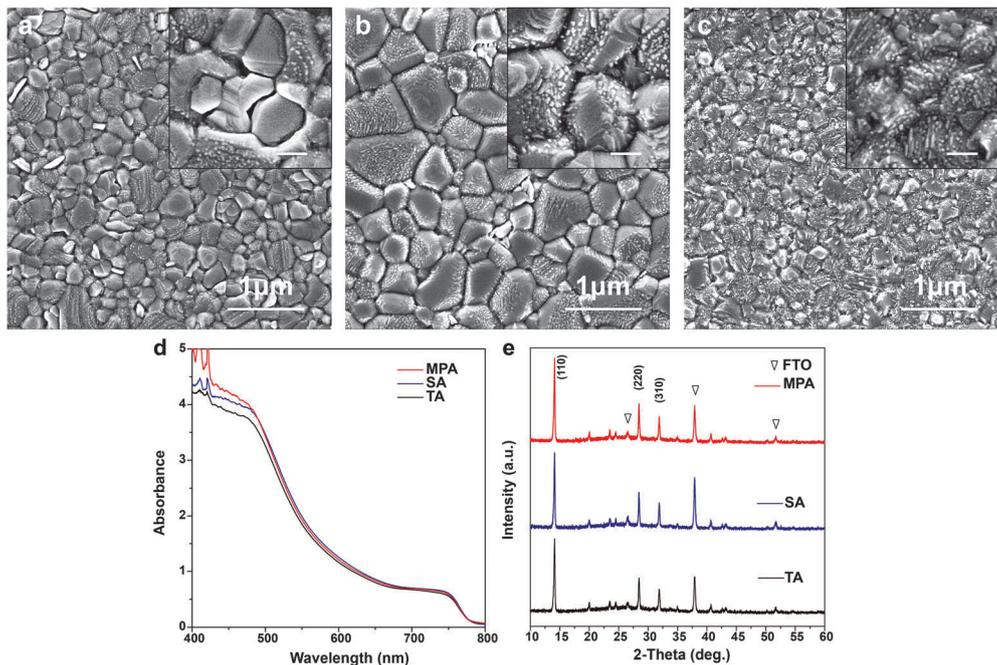
Fig. 2 SEM images of the MAPbI<sub>3</sub> perovskite films with thermal annealing (a), DMF solvent annealing (b) and methylamine post-annealing (c) treatments. High-magnification SEM images are shown in the insets, with scale bars representing 200 nm. UV-vis spectra (d) and XRD patterns (e) of MAPbI<sub>3</sub> films with various post-annealing treatments. Methylamine post-annealing promotes greater continuity between adjacent grains, compared to solvent and thermal annealing.
