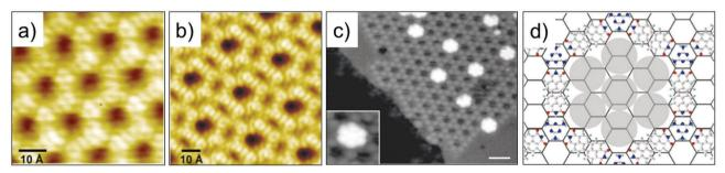
Fig. 1 Early examples of host-guest systems. STM images of the (a) Chicken wire and (b) flower structure of TMA self-assembled network on HOPG. (c) STM image showing entrapment of heptameric C<sub>60</sub> clusters in the PTCDI-melamine host network assembled on Ag terminated silicon surface. (d) Schematic of the PTCDI-melamine host-guest system. Reproduced from ref. 30 and 31 with permission from Wiley-VCH and Macmillan Publishers Ltd, respectively.
