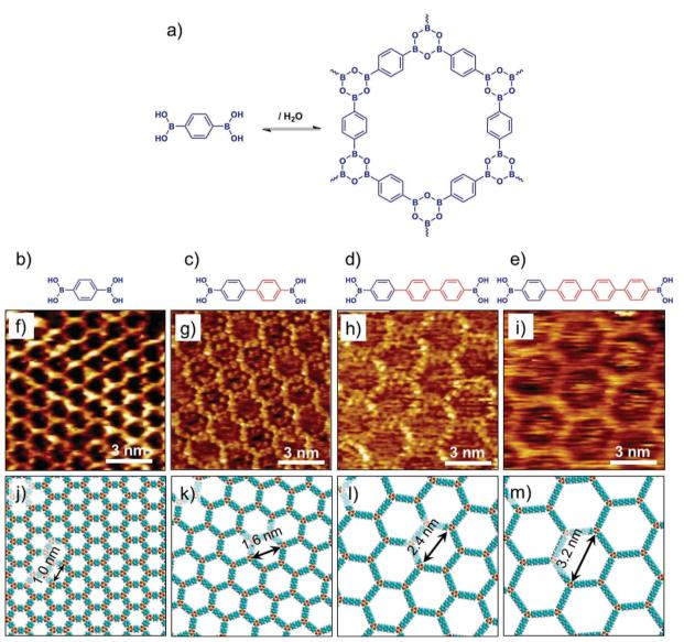
Fig. 6 Surface synthesis of isoreticular 2D-COFs. (a) A reaction scheme showing boronic acid self-condensation to yield boroxine based COF. (b-e) Molecular structures of the boronic acid building blocks with increasing length of the oligophenylene backbone. (f-i) Corresponding STM images of 2D-COF films synthesized on graphite surface. (j-m) Molecular models of the isoreticular COF networks. Reproduced from ref. 72, 73 with permission from the American Chemical Society
