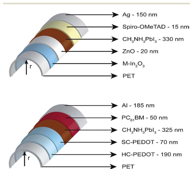
Fig. 1 Schematic of the device architecture for M-In<sub>2</sub>O<sub>3</sub>/ZnO/CH<sub>3</sub>NH<sub>3</sub>PbI<sub>3</sub> (top) and HC-PEDOT/SC-PEDOT/CH<sub>3</sub>NH<sub>3</sub>PbI<sub>3</sub> (bottom) cells, bent at a radius of curvature,  $r$ .
