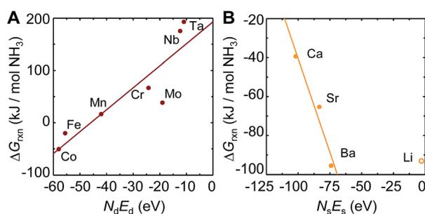
Fig. 2 Scaling of the free energy of the NH<sub>3</sub> evolution at 25 °C (computed from tabulated free energy data as described in Section 3.1) via metal nitride (A) reduction and (B) hydrogenation with the product of the number of electrons in the metal ground state,  $N$ , and the energy of these electrons,  $E$ , in the (A) d-states and (B) s-states. The metal marks the metallic constituent of the composition given with ESI.† Solid lines are fits to the data shown with solid symbols.
