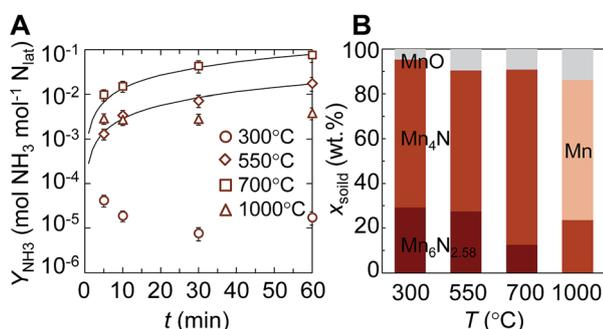
Fig. 6  $\text{NH}_3$  evolution *via* isothermal transition-metal nitride reduction: (A)  $\text{NH}_3$  yield vs. time and (B) solid weight fractions from the reaction of  $\text{Mn}_4\text{N}$  with  $\text{H}_2$  at 1 bar vs. temperature. Error bars are *via* error propagation within a 95% confidence interval. Solid lines are shrinking-core models for the data at 550 °C and 700 °C controlled by the chemical reaction or gas phase diffusion.
