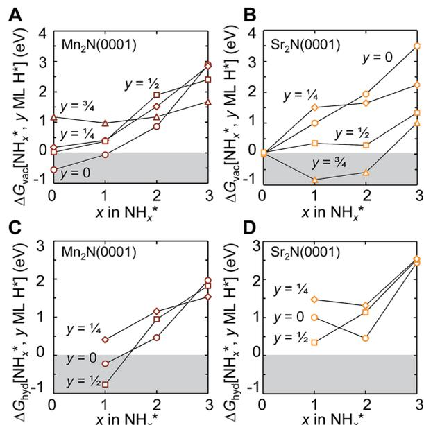
Fig. 3 Free energy diagrams for (A and B) forming  $1/4$  ML  $v_N$  yielding  $1/4$  ML  $NH_x^*$  and (C and D) hydrogenating  $NH_{x-1}^*$  to  $NH_x^*$  and  $y = 0$  (circles),  $1/4$  (diamonds),  $1/2$  (squares), and  $3/4$  (triangles) ML  $H^*$  adatoms on (A and C)  $Mn_2N(0001)$  and (B and D)  $Sr_2N(0001)$  at  $25^\circ C$  and 1 bar. Lines are a guide only. The shaded regions mark energetically favourable surface reactions.
