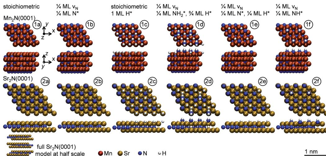
Fig. 5 Optimized adsorption geometries for the indicated surface conditions (top two lines) of (1a to 1f)  $\text{Mn}_2\text{N}(0001)$  and (2a to 2f)  $\text{Sr}_2\text{N}(0001)$ . The view along the  $y$ -axis of the  $\text{Sr}_2\text{N}(0001)$  model is limited to the upper layer.
