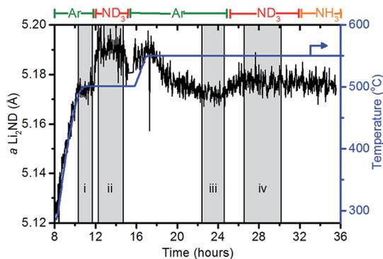
Fig. 6 Variation of the  $a$  lattice parameter of  $\text{Li}_2\text{ND}$  (black) over the course of the experiment. The temperature of the sample (blue) is shown for comparison. Shaded areas represent periods of NPD data which were summed and analysed for the sample stoichiometry.
