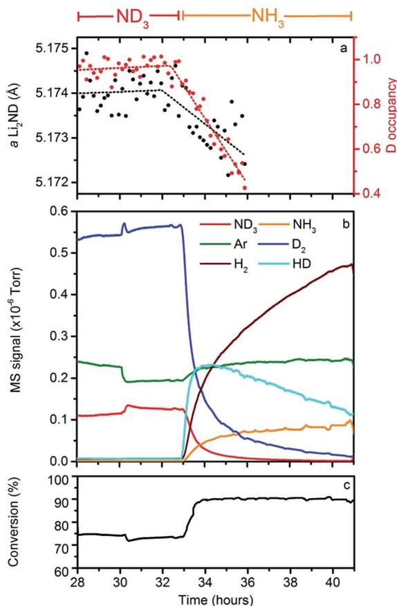
Fig. 7 H–D exchange experiment, where the gas species flowing across the sample during the experiment are shown at the top. The panels show (a) the refined deuterium occupancy (red) and lattice parameter (black) in the  $\text{Li}_2\text{ND}$  sample, (b) the QGA data collected during the experiment and (c) the ammonia conversion percentage data.
