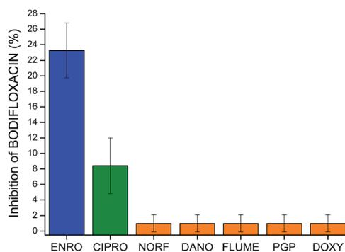
Fig. 7 Inhibition of BODIFLOXACIN (%) for MIPs incubated with ENRO, CIPRO and other antibiotics. Incubation conditions: 250 nM BODIFLOXACIN, 10  $\mu M$  of ENRO or interfering substances, 60 minutes in 50 : 50 (v/v) MeCN : HEPES (25 mM pH 7.5),  $n = 3$ . Measurements performed via imaging.
