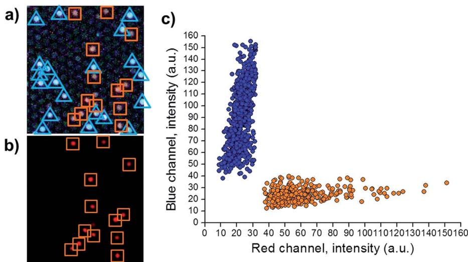
Fig. 3 Micrographs that show (a) fluorescence of coumarin-30 and  $[\text{Ru}(\text{dip})_3]\text{Cl}_2$  exciting at 405 nm, and (b) fluorescence of  $[\text{Ru}(\text{dip})_3]\text{Cl}_2$  exciting at 470 nm. (c) Population distribution intensities of red and blue channels of MIP (encoded with coumarin-30, blue points,  $n = 734$ ) and NIP (encoded with  $[\text{Ru}(\text{dip})_3]\text{Cl}_2$ , orange points,  $n = 382$ ) microspheres.
