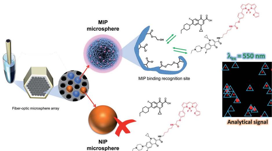
**Fig. 2** Workflow of the assay protocol. ENRO quantification was based on a competitive assay in which the target analyte competes with the labeled ENRO (BODIFLOXACIN) to bind to specific binding sites on the MIP microspheres.
