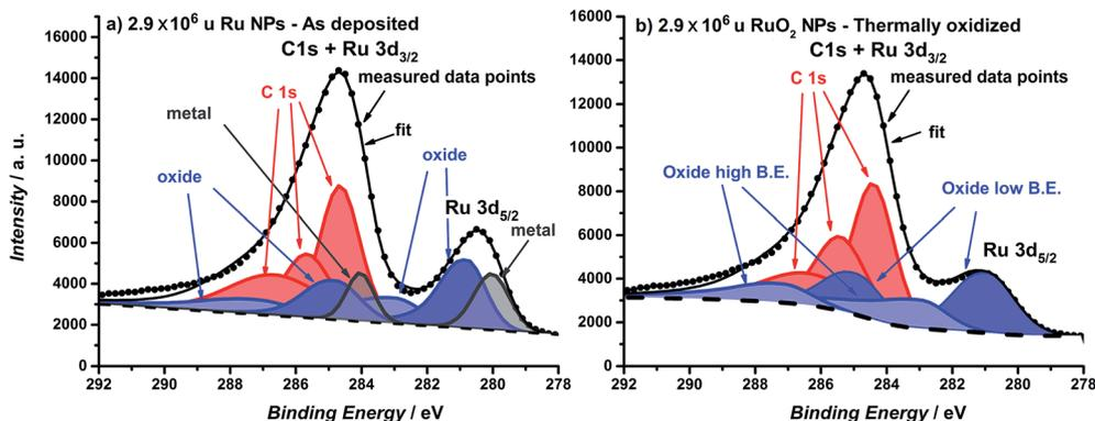
Fig. 1 XPS spectra of the Ru 3d core level region of (a) as-deposited  $2.9 \times 10^6$  u Ru nanoparticles and (b) thermally oxidized  $2.9 \times 10^6$  u RuO<sub>2</sub> nanoparticles. Ruthenium oxide is fitted with two species and carbon is fitted with three species. For further details about the fitting see the ESI.†
