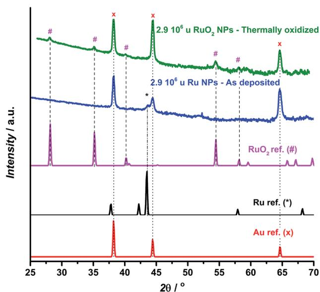
Fig. 2 GA-XRD for as deposited (blue) and thermally oxidized (green)  $2.9 \times 10^6$  u ruthenium nanoparticles deposited on a Au(111) single crystalline substrate, together with reference patterns for Au,<sup>53</sup> Ru<sup>54</sup> and RuO<sub>2</sub>.<sup>55</sup>
