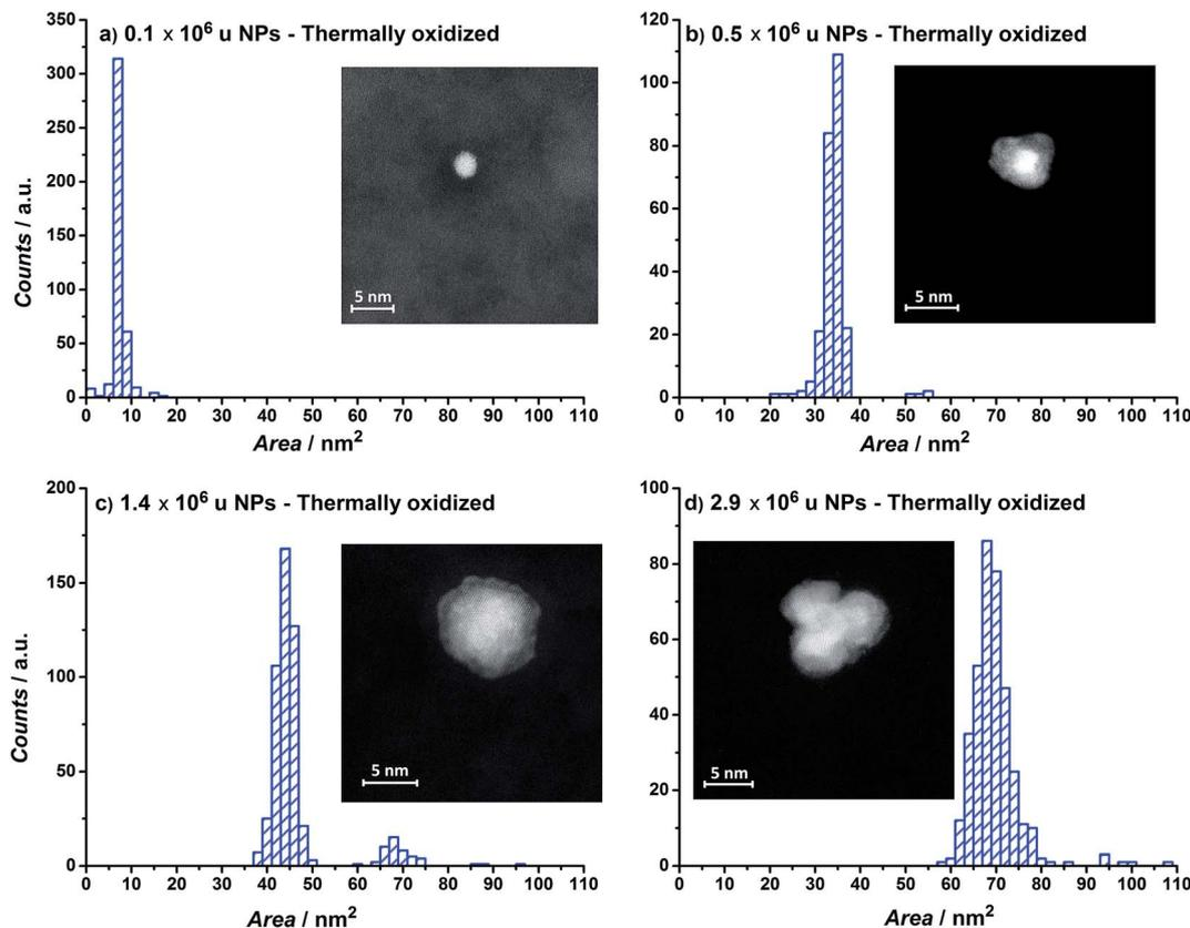
Fig. 3 Nanoparticle area distributions and HAADF-Scanning Transmission Electron Microscopy images of thermally annealed  $\text{RuO}_2/\text{Si}_3\text{N}_4$  samples for particle mass of (a)  $0.1 \times 10^6$ , (b)  $0.5 \times 10^6$ , (c)  $1.4 \times 10^6$  and (d)  $2.9 \times 10^6$  u.
