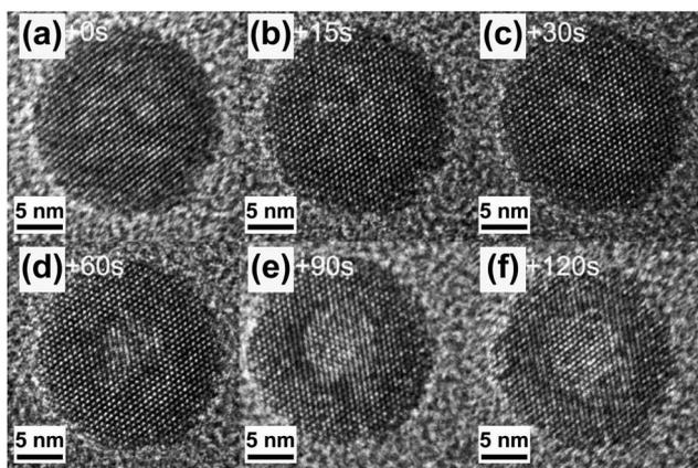
Fig. 7 Morphologic evolution of a hexagonal-phase  $\text{NaYF}_4\text{:Yb/Er}$  (20/2 mol%) nanocrystal under electron beam irradiation at different time intervals. (a–f) 0, 15, 30, 60, 90 and 120 s, respectively. (Reprinted with permission from ref. 131. Copyright 2009, Wiley-VCH Verlag GmbH & Co. KGaA.)
