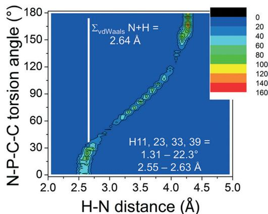
Fig. 2 Plot of the absolute N–P–C–C torsion angle vs. the *ortho*-C–H $\cdots$ N distances found in 1315  $[\text{PPN}]^+$  structures found within 1120 CIFs. The numbers indicated in white are taken from the X-ray structure of **1** highlighted in this work.
