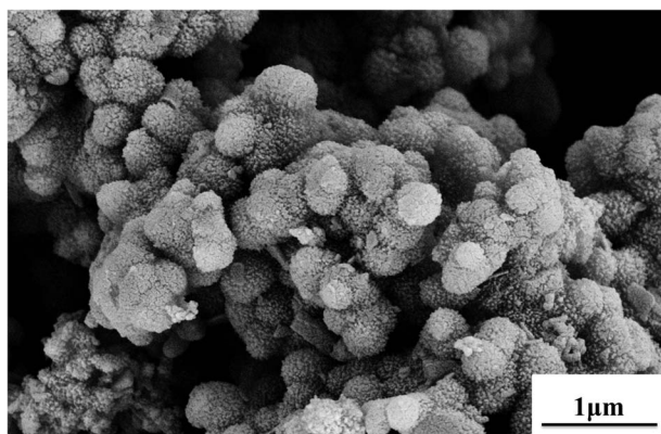
Fig. 6 SEM images of PANI nanosphere prepared in phosphoric acid. Synthetic conditions: [aniline] = 0.2 M, [aniline]–[APS] = 4 : 5, [H 3 PO 4 ] = 1 M.
