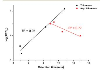
Fig. 7 The relationship between retention time (determined by C18 HPLC) and transport activity of thioureas 1-4 and acylthioureas 5-8 as determined by an ISE assay.
