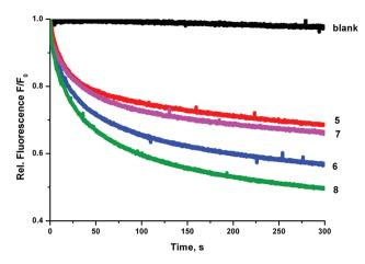
Fig. 6 Chloride influx mediated by receptors 5-8 (preincorporated at 0.5 mol% with respect to lipid) into vesicles containing 225 mM NaNO<sub>3</sub> buffered to pH 7.2 with sodium phosphate salts and 1 mM lucigenin. The vesicles were suspended in 225 mM NaNO<sub>3</sub> and the experiment was initiated by adding 25 mM NaCl. Each experiment was repeated in triplicate.
