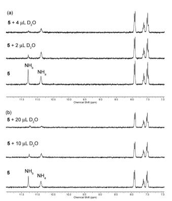
Fig. 3 Changes to the downfield region of the <sup>1</sup>H NMR spectrum of receptor 5 (5 mL of 0.01 M solution) in (a) DMSO-d<sub>6</sub> and (b) DMSO-d<sub>6</sub> with 1% H<sub>2</sub>O (v/v) upon the addition of D<sub>2</sub>O.
