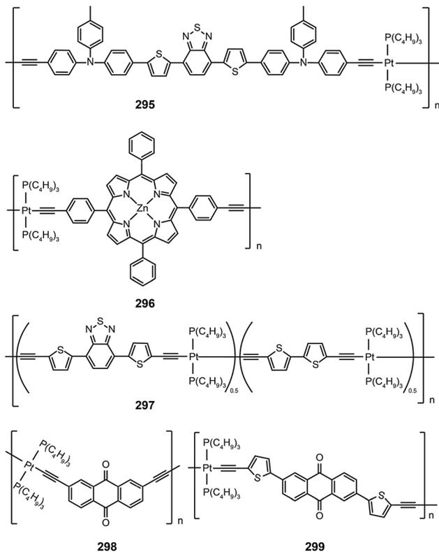
Several other groups have also made significant contributions to development of Pt(II)-based complexes for OPVs. Li *et al.*<sup>165</sup> prepared a solution-processable acetylide polymer (**298**) functionalized with an electron-deficient anthraquinone
