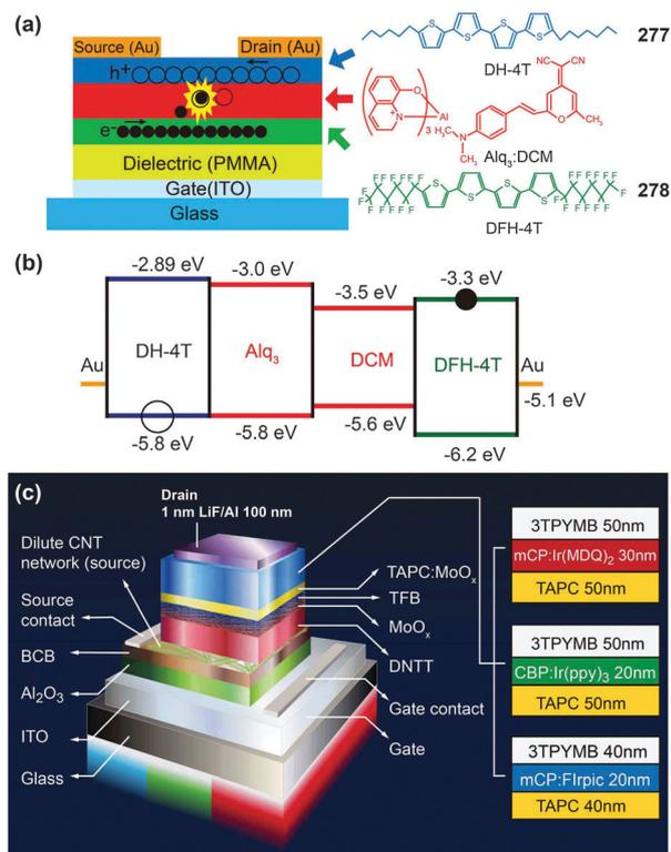
**Fig. 21** (a and b) Device configuration and energy level scheme of a trilayer OLET using Alq<sub>3</sub>:DCM, DH-4T and DFH-4T as emitting, hole-transporting, and electron-transporting layers, respectively. (c) Device structures of a trilayer OLET with direct integration of red, green and blue OLED and OTFT. (Reproduced with permission from ref. 8 and 121. Copyright 2011 and 2010, respectively, American Association for the Advancement of Science and Nature Publishing Group.)
