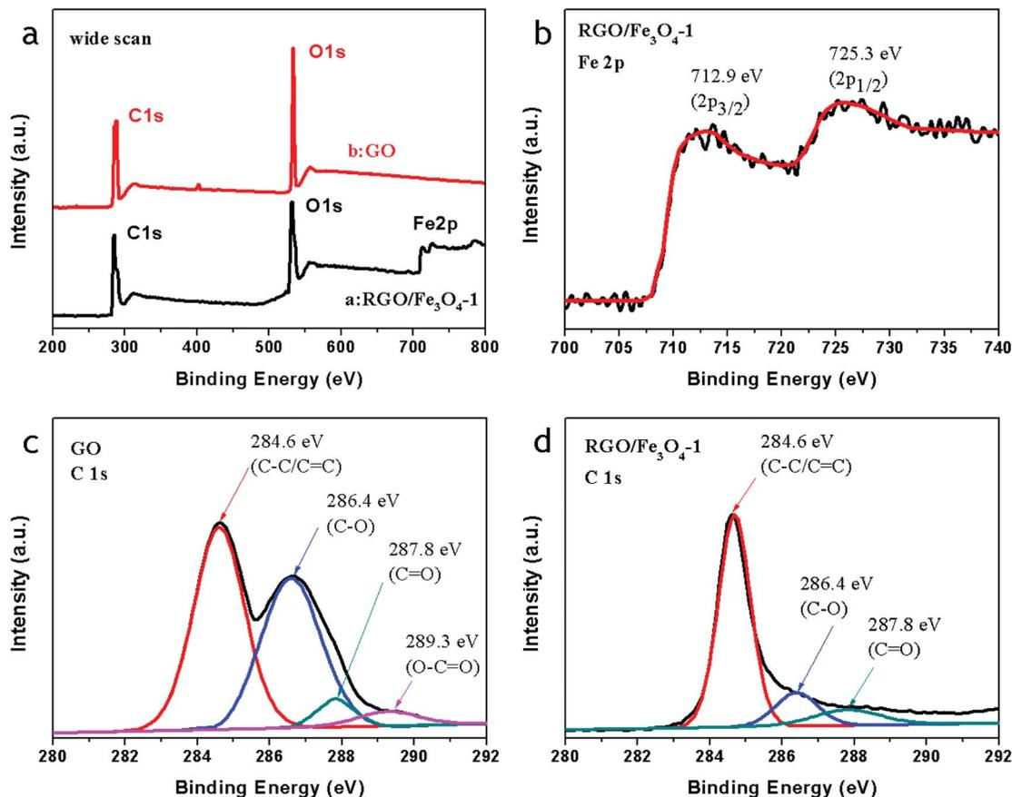
Fig. 3 X-ray photoelectron spectroscopy (XPS) spectra: wide scan (a), Fe 2p spectrum of the RGO- $\text{Fe}_3\text{O}_4$ -1 composite (b), C 1s spectrum of RGO (c), and C 1s spectrum of the RGO- $\text{Fe}_3\text{O}_4$ -1 composite (d).
