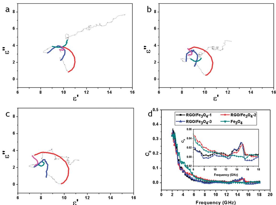
**Fig. 9**  $\epsilon'$ – $\epsilon''$  curves of RGO–Fe<sub>3</sub>O<sub>4</sub>-1 composite (a), RGO–Fe<sub>3</sub>O<sub>4</sub>-2 composite (b) and RGO–Fe<sub>3</sub>O<sub>4</sub>-3 composite (c);  $C_0$ – $f$  curves of Fe<sub>3</sub>O<sub>4</sub> NPs and RGO–Fe<sub>3</sub>O<sub>4</sub> composites (d), inset is the expansion of the curves.
