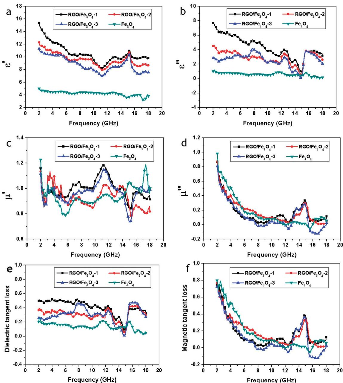
**Fig. 8** Frequency dependence on real parts (a) and imaginary parts (b) of the complex permittivity, real parts (c) and imaginary parts (d) of the complex permeability, and the corresponding dielectric loss tangents (e) and magnetic loss tangents (f) of  $\text{Fe}_3\text{O}_4$  and RGO- $\text{Fe}_3\text{O}_4$  composites.
