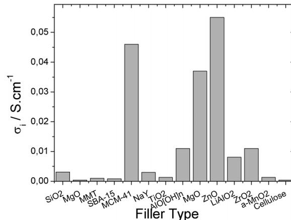
Fig. 4 Ionic conductivity for different filler types.
